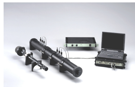
Fig. 2 Normal Incidence Transmission Loss measurement System
